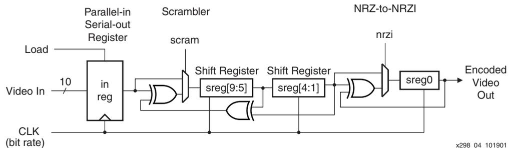
Figure 4: Bit-rate Serial SDI Scrambler
