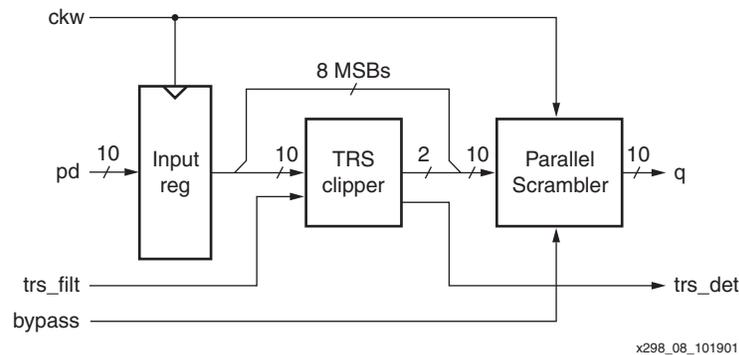
Figure 8: X7C9235 Example Block Diagram
