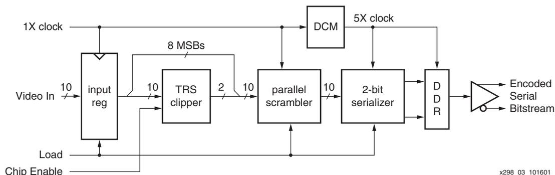
Figure 3: Example SDI Transmitter with TRS Clipper
