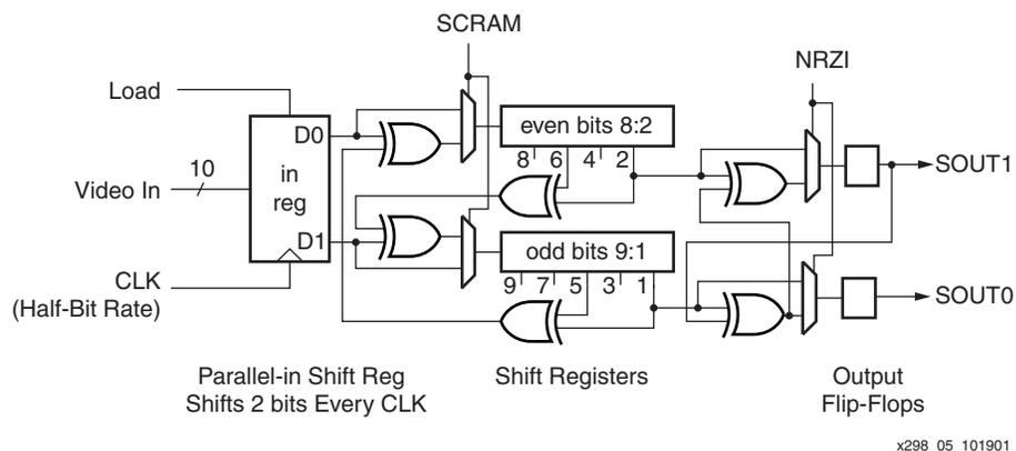
Figure 5: SDI Scrambler Processing Two Bits Per Clock Cycle
