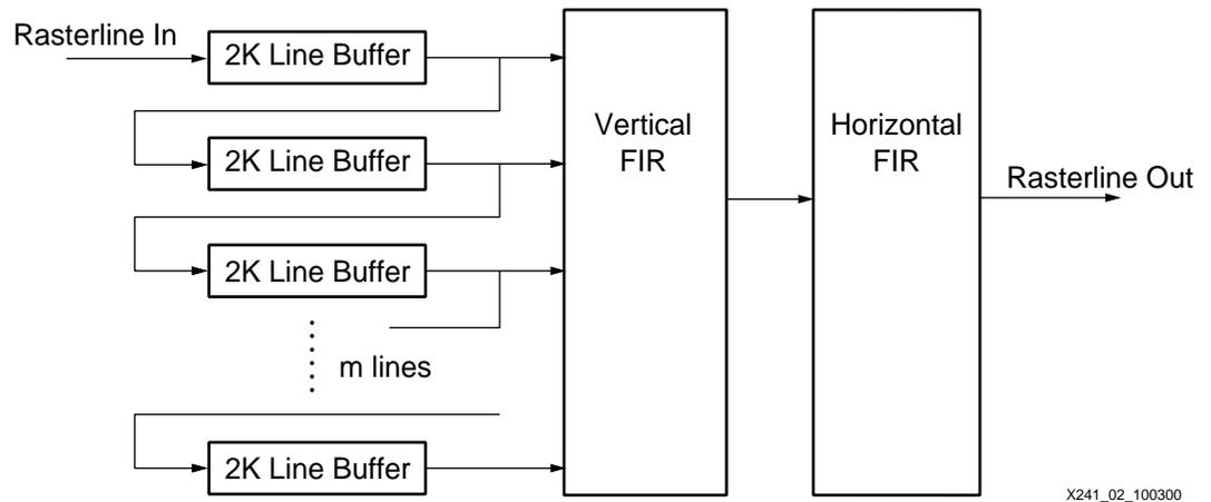
Figure 2: 2D FIR Filter With Built-in Line Buffers
