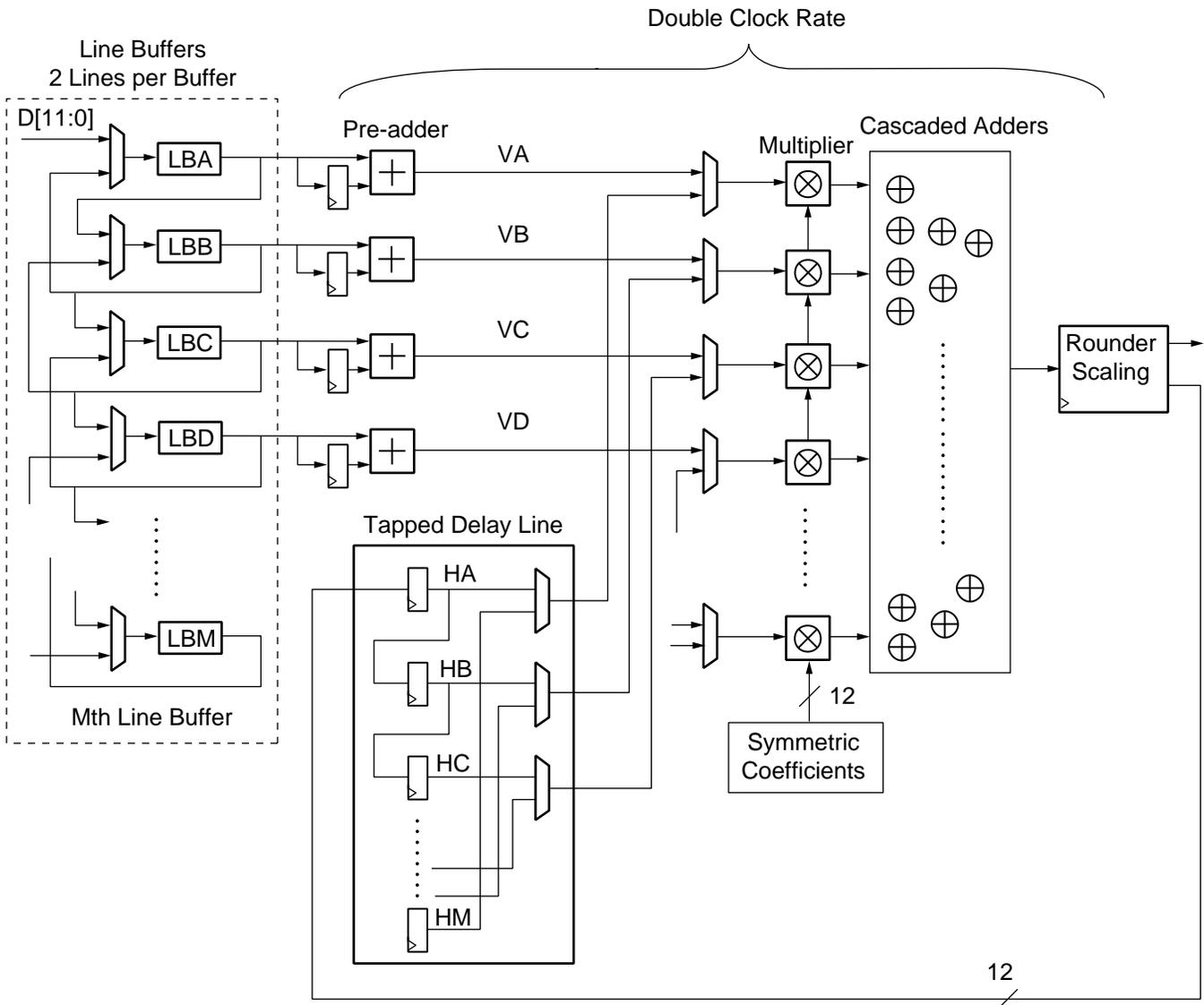
Figure 5: 2D FIR Algorithm
