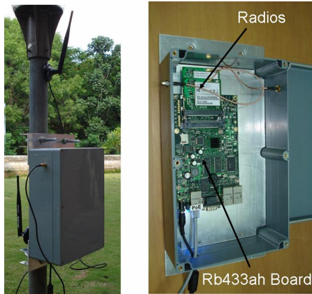
Figure 3. Installed Mesh Node & Mesh Node Internals
