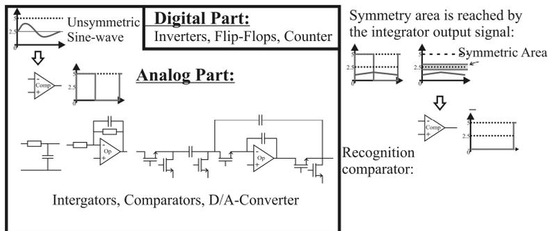
**Figure 3. Load-symmetry recognition circuit principle of a sine-wave**
