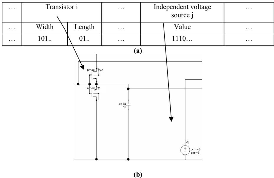
**Figure 2. a) Chromosome and b) the parameters of the circuit elements, created from it**
