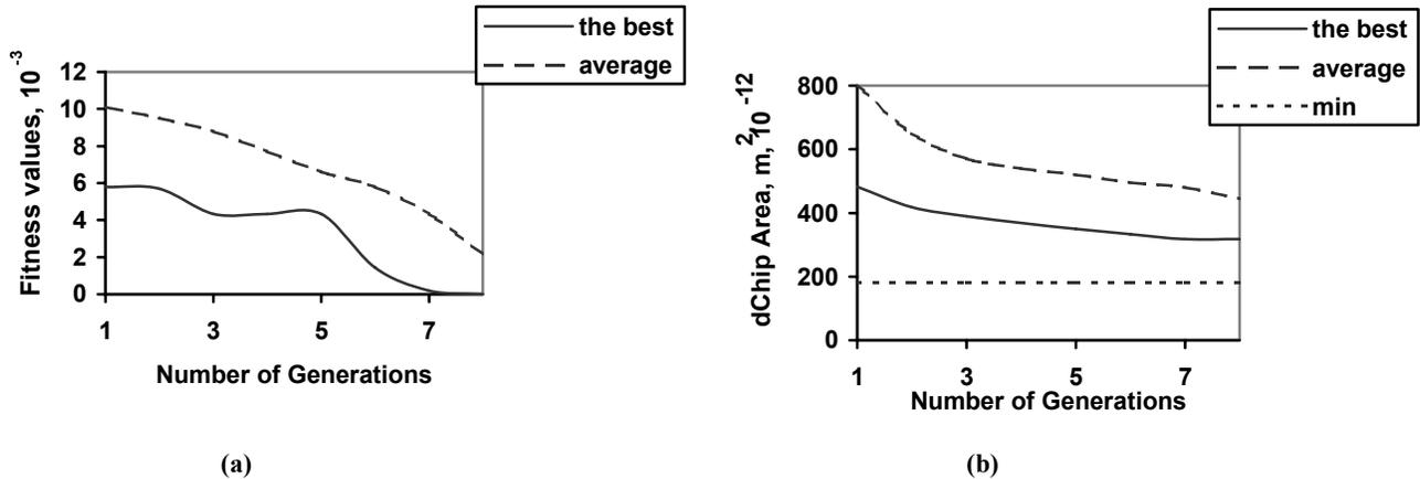
**Figure 4. Performance (average of 10 runs) behaviour of classical UMDA for population size  $N=4$  and truncation selection with  $\tau=0.5$  a) for deviations of symmetry recognition b) for chip area variations in microns.**
