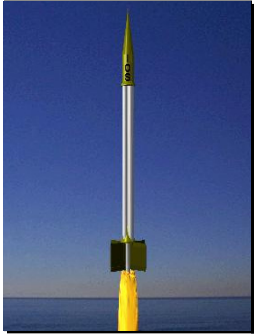
Fig. 1. The Interorbital Systems RSX-2 Rocket. The RSX-2 is capable of lifting a 5 pound payload into the upper atmosphere using a cluster of four liquid-fueled thrusters. It is currently the only liquid-fueled sounding rocket in production. Such rockets are desirable because of their low acceleration rates and non-corrosive exhaust products.
