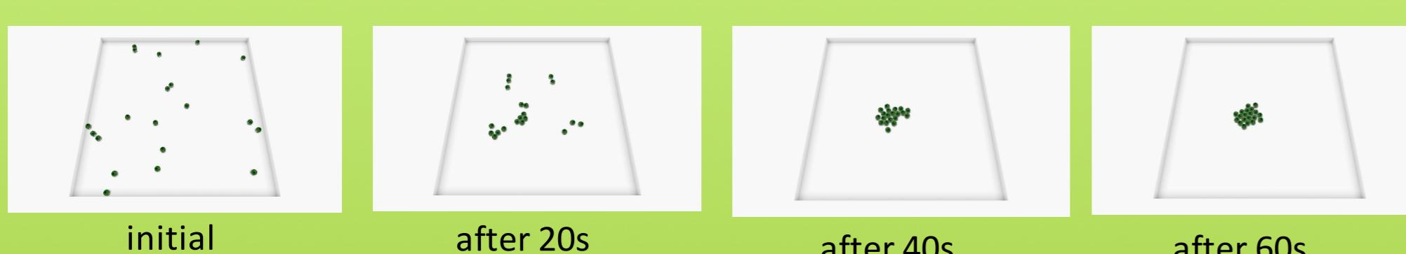
Snapshots of the aggregation behaviour of 20 e-puck robots in Enki simulation, using the automatically generated controller code from RoboChart
