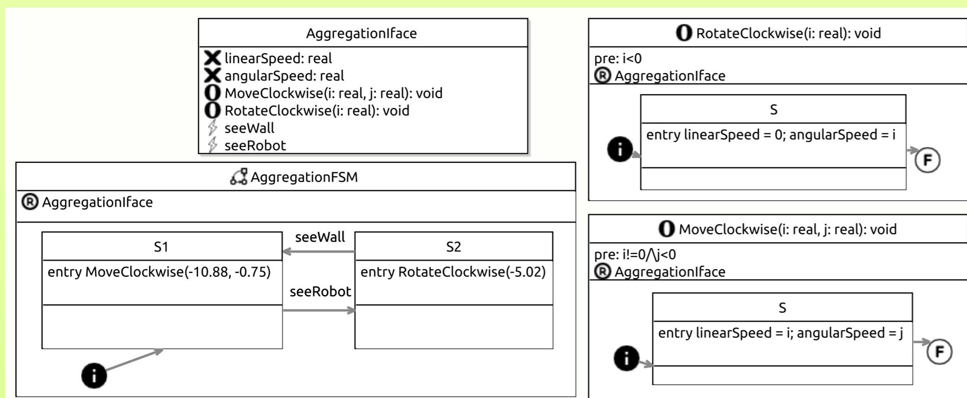
Diagram of the aggregation controller modelled in RoboChart
