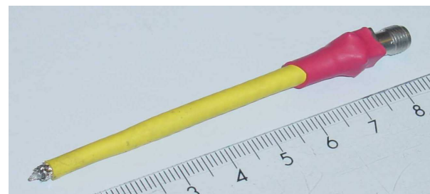
Figure 4. H-field probe for the surface scan method.
