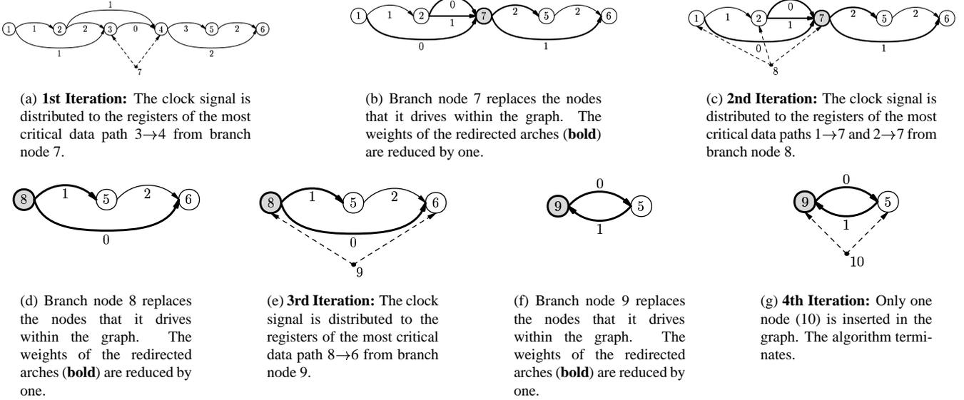
Figure 4. Iterations of the algorithm to reduce the input graph to a single node.
