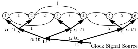
(a) Binary clock tree topology for an arbitrary circuit
