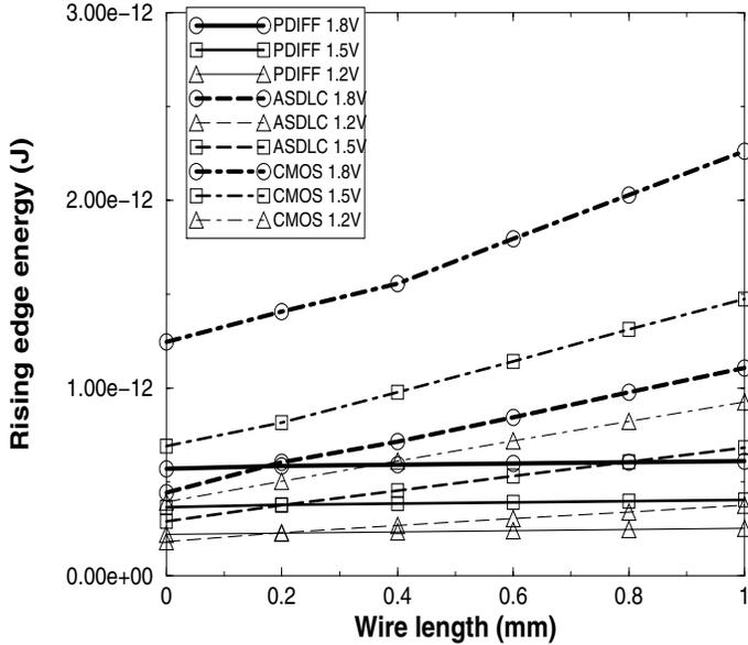
Figure 7: Rising edge energy for a metal2 wire.  $V_{ref}=0.3V$ .
