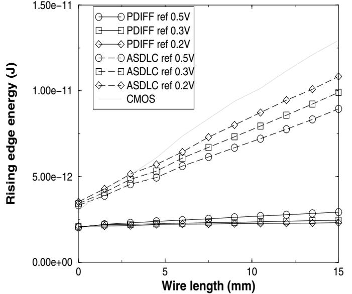
Figure 8: Rising edge energy for a metal5 wire.  $V_{dd}=1.8V$ .
