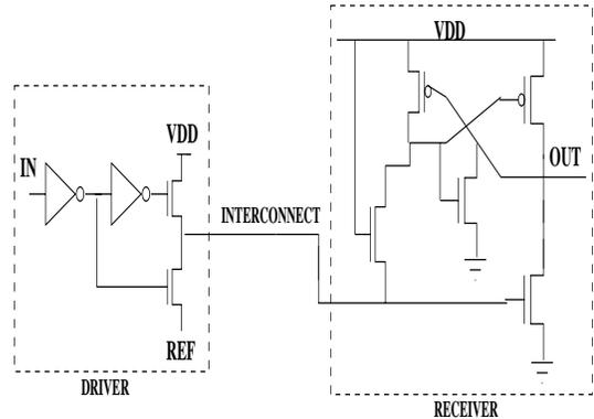
Figure 2: Asymmetric source-follower driver with level converter
