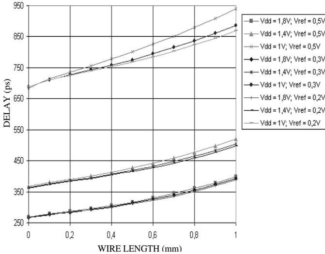
Figure 5: PDIFF scheme delay as a function of  $L$ ,  $V_{dd}$  and  $V_{ref}$
