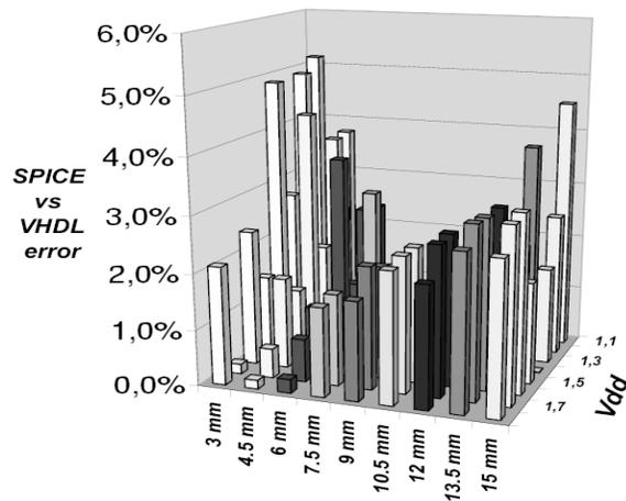
**Figure 9: Percentage error between VHDL estimation and SPICE simulation for a bus line traced waveform**
