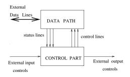
Figure 1. CP-DP Partition in the Circuit Structure
