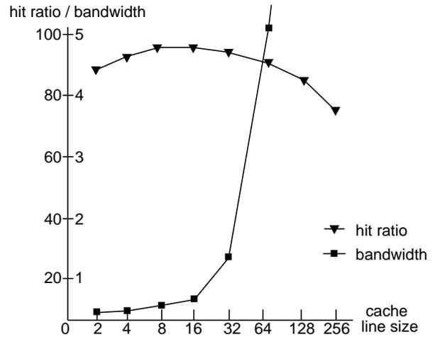
Figure 2. The cache hit ratio and memory bandwidth variation with the cache line size for the go benchmark
