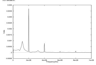
Figure 8. FFT of transient voltage of a 200MHz PowerPCtm
