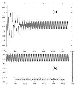
Figure 7. Transient analysis starting from (a) DC solution and (b) estimated steady state solution
