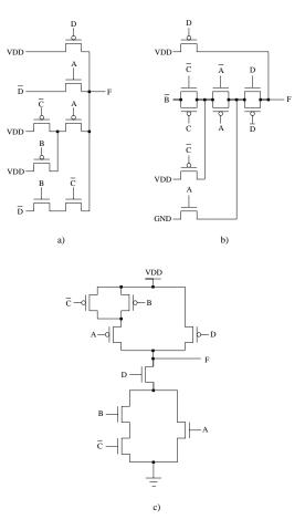
Figure 5: Function  $F = \overline{D} + \overline{A}\overline{B} + \overline{A}C$  synthesized in a) HPGL, b) PGL, c) CMOS
