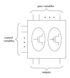
Figure 1: General structure of a pass transistor network
