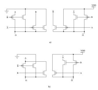
Figure 2: Example of AND/NAND gate implementation in a) DPL, b) DVL
