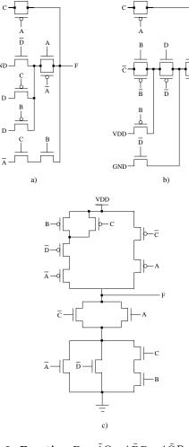
Figure 6: Function  $F = \overline{A}C + A\overline{B}D + A\overline{C}D$  synthesized in a) HPGL, b) PGL, c) CMOS
