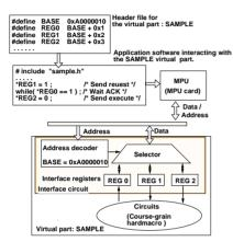
Figure. 8. Interaction between the virtual part and the application software.
