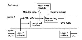
Figure. 10. A block diagram of the implemented dynamic VC switch.
