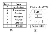
Figure. 1. Open system interconnection (OSI) reference model (A) and an implemented application structure (B).
