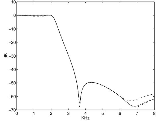
Figure 2: The time-sampled switched-capacitor filter transfer function.
