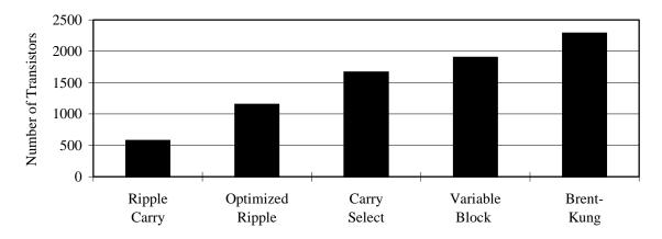
Figure 10. The transistor counts of the Basic Ripple, Optimized Ripple, Carry Select, Variable Block, and Brent-Kung carry chains.
