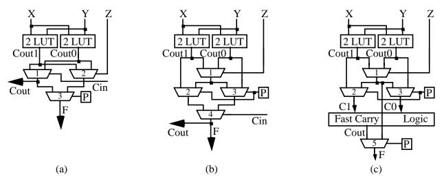
Figure 2. Carry computation elements with faster carry propagation.
