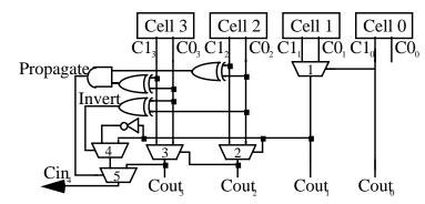
**Figure 4.** The Variable Block carry structure. Mux 1 performs an initial two stage ripple carry. Muxes 2 through 5 form a 2-bit Variable Block block. Mux 5 decides whether the Cin signal should be sent directly to Cout, while mux 4 decides whether to invert the Cin signal or not.
