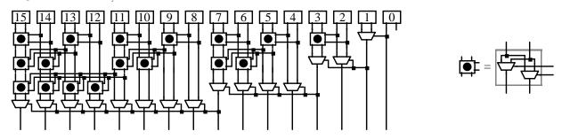
**Figure 5.** The 16 bit Brent-Kung structure. At right is the details of the concatenation block. Note that once the Cin has been computed for a given stage, a mux is used in place of a concatenation block.
