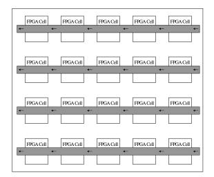
**Figure 11.** The location of the carry chains within the FPGA.
