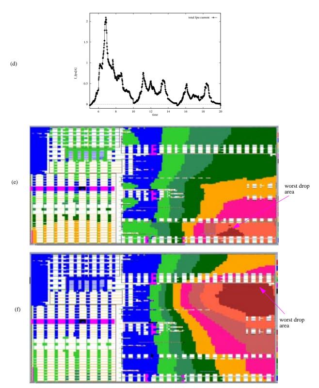
Fig. 3. PPC<sup>TM</sup> 750 case study: (a) power grid and block layout, (b) voltage map for area-based block currents, (c) voltage map inside the FPU for area-based block currents, (d) total transient currents in the FPU, (e) voltage map inside the FPU for total current of 0.7A, (f) voltage map inside the FPU for total current of 2.1A.
