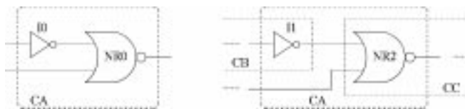
(a) One subcircuit in the schematic (b) The subcircuit in the layout
