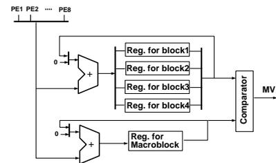
Figure 6: Block diagram of accumulator.
