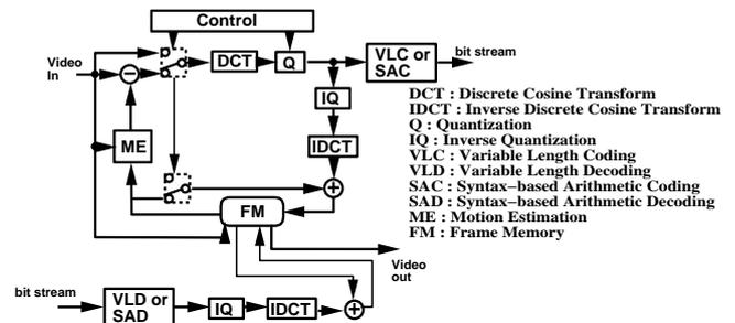
Figure 1: H.263 encoding/decoding process.
