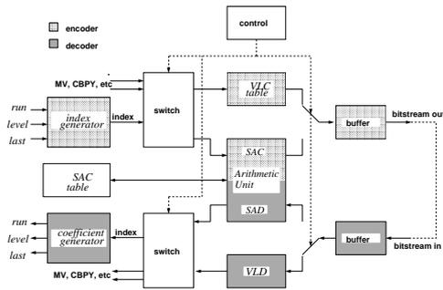
Figure 11: Block diagram of VLC/VLD and SAC/SAD core.
