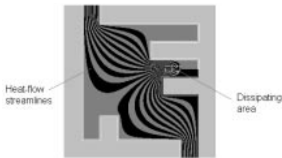
Fig. 13. Streamlines of the heat-flow
