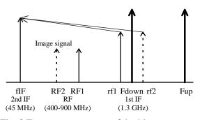
Fig. 3 Frequency spectrum of double-super tuner
