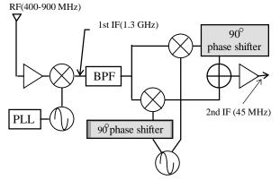
Fig 4. Block diagram of double-super tuner with image rejection mixer
