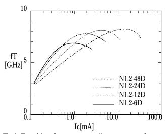
Fig.9 Transition frequency vs collector current for npn transistors.
