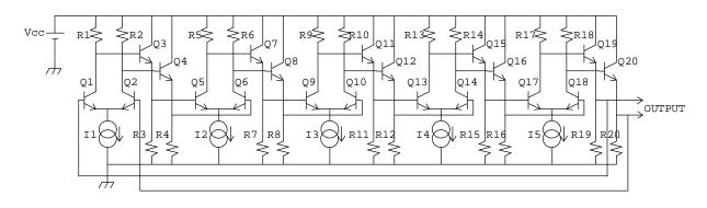
Fig. 11 Five stage ring oscillator
