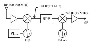
Fig 2. Block diagram of double-super tuner
