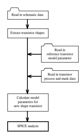
Fig. 10 Flow diagram for transistor model parameter generation program for various transistor shapes
