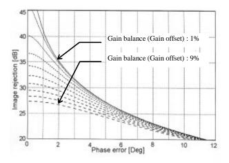
Fig. 5 AHDL simulation result of image rejection tuner
