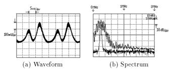
Fig. 6. Noises from a HF lamp
