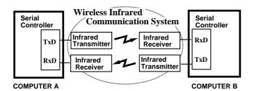
Fig. 2. Serial communication system by wireless infrared communication  $% \left( {{{\rm{S}}_{{\rm{s}}}}} \right)$
