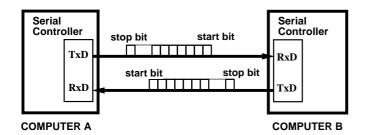
Fig. 1. Serial communication system
