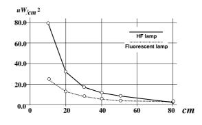
Fig. 5. Intensity of optical noise from lamps
