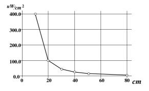
Fig. 7. Signal intensity at photo detector
