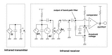
Fig. 10. Model of infrared communication
