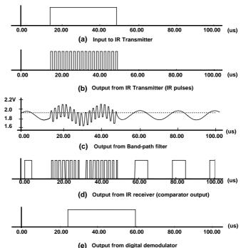
Fig. 11. Outputs of infrared receiver with modeled noises
