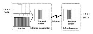
Fig. 3. Amplitude Shift Keying
