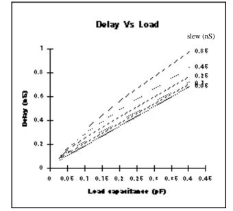
Figure 8: Delay variation with load capacitance and input slew.
