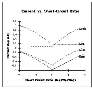
Figure 3: Peak current variation with dynamic short-circuit ratio.
