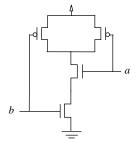
Figure 7: Nand gate example shown in Table 1.
