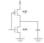
Figure 2: Inverter for characterizing charge and current.
