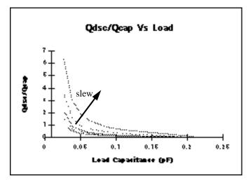
Figure 1: Ratio of dynamic short-circuit charge to capacitive charge as a function of load capacitance and input slew. For large slew and small capacitance the dynamic short-circuit charge exceeds the capacitive charge.
