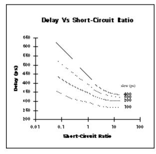
Figure 9: Variation of delay with short-circuit ratio for different input slew and fixed load capacitance.
