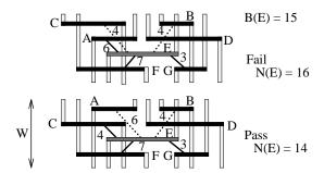
Figure 2: Crosstalk Avoidance Channel Routing
