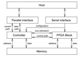
Figure 1: Overall structure of the board
