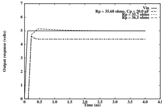
**FIGURE 13:** Output response of a low-loss line with parallel AC termination in contrast with parallel resistance termination. OTTER yields values of  $R_p=35.68 \Omega$  and  $C_p=20.0 \text{ pF}$  using the symbolic analysis approach described.  $R_{\text{line}}=5.0 \Omega$ .
