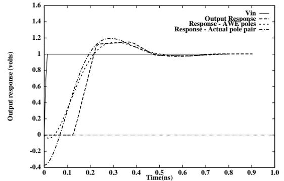
**FIGURE 6:** Time domain response of a low-loss transmission line with a capacitive load of 0.1pF,  $r=0.13 \Omega/\text{mm}$ ,  $l=0.2\text{nH/mm}$ ,  $c=0.15\text{pF/mm}$ ,  $length=25\text{mm}$ ,  $Z_0=36.51$ ,  $T_f=0.14\text{ns}$ .
