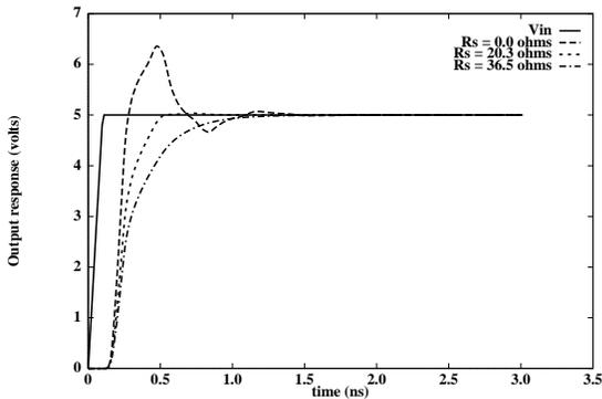
**FIGURE 9:** Time-domain response for lossy transmission line ( $Z_0 = 36.51 \Omega$ ,  $R_{line} = 40 \Omega$ ) with termination value  $R_s = 0.0 \Omega$ ,  $20.3 \Omega$  (termination value from  $m_3$ ) and  $36.5 \Omega$ .
