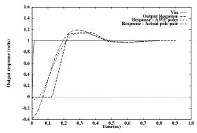
**FIGURE 6:** Time domain response of a low-loss transmission line with a capacitive load of 0.1pF. r=0.13  $\Omega$  /mm, t=0.2nH/mm, c=0.15pF/mm. length=25mm,  $Z_0$ =36.51,  $T_f$ =0.14ns.
