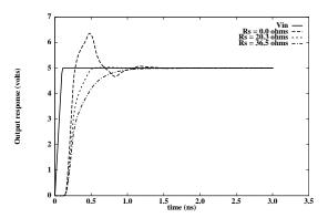
**FIGURE 9:** Time-domain response for lossy transmission line ( $Z_0 = 36.51 \Omega$ ,  $R_{\rm line} = 40 \Omega$ ) with termination value  $R_{\rm s} = 0.0 \Omega$ , 20.3  $\Omega$  (termination value from  $m_3$ ) and 36.5  $\Omega$ .
