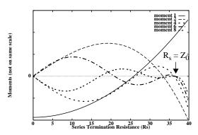
**FIGURE 2:** Moments  $m_1, m_2, m_4, m_6$  and  $m_8$  of the voltage response  $V_2$  as a function of the termination resistance,  $R_s$ .  $Z_0$ =36.5  $\Omega$
