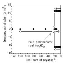
**FIGURE 4:** Movement of first pole-pair as a function of the termination resistance  $R_s$ . Pole-pair becomes real for  $R_s = Z_0$ .
