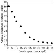
**FIGURE 7:** Optimal termination resistance  $(R_{\text{opt}})$  as function of capacitive load  $(C_{\text{L}})$ .  $C_{\text{line}}$ =3.75pF. For  $C_{\text{L}}$ < $C_{\text{line}}$ ,  $R_{\text{opt}}$ = $Z_{\text{0}}$ .
