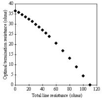
**FIGURE 8:** Optimal termination resistance,  $R_s$ , plotted as a function of the resistance of the transmission line,  $R_{line}$ .  $Z_0=36.5\,\Omega$ . Self termination condition for the line is  $R_{line}=109.5\,\Omega$ .
