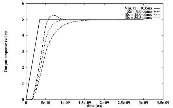
**FIGURE 11:** Output response of lossy line ( $R_{line} = 60.0 \Omega$ ,  $Z_0 = 36.51 \Omega$ ) for input signal rise-time,  $t_r = 0.35$  ns.  $R_s = 0.0 \Omega$  (optimal series termination resistance obtained from moment-3),  $R_s = 15.0 \Omega$  (from moment-6) and  $R_s = 36.5 \Omega$  ( $Z_0$ ).
