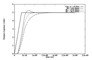
**FIGURE 11:** Output response of lossy line ( $R_{\rm line}$ =60.0  $\Omega$ ,  $Z_0$ =36.51  $\Omega$ ) for input signal rise-time,  $t_{\rm r}$ =0.35ns.  $R_{\rm s}$ =0.0  $\Omega$  (optimal series termination resistance obtained from moment-3),  $R_{\rm s}$ =15.0  $\Omega$  (from moment-6) and  $R_{\rm s}$ =36.5  $\Omega$  ( $Z_0$ ).
