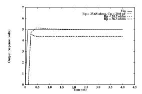
**FIGURE 13:** Output response of a low-loss line with parallel AC termination in contrast with parallel resistance termination. OTTER yields values of  $R_{\rm p}{=}35.68\,\Omega$  and  $C_{\rm p}{=}20.0{\rm pF}$  using the symbolic analysis approach described.  $R_{\rm line}{=}5.0\,\Omega$ .
