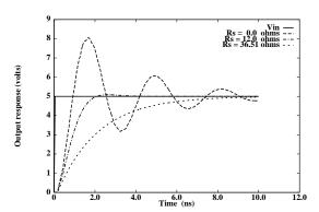
**FIGURE 3:** Output response of low-loss line  $(Z_0=36.51\,\Omega)$  with capacitive load  $(C_1)$  and optimal series termination resistance  $(R_s)$  obtained using  $m_3$  via symbolic analysis.  $C_1=50.0$ pF.
