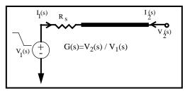
**FIGURE 1:** Open circuited lossless line with series termination at source end. l=0.2nH/mm, c=0.15pF/mm, length=25mm,  $Z_0$ =36.51,  $T_f$ =0.14ns.
