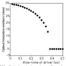
**FIGURE 10:** Optimal termination resistance,  $R_{\rm opt}$ , as function of input signal rise-time,  $t_{\rm r}$ .  $T_{\rm f}$  = 0.14ns.  $R_{\rm opt}$  obtained from moment analysis (using  $m_3$ ) equals  $\theta$  for  $t_r \approx 2T_f$ .
