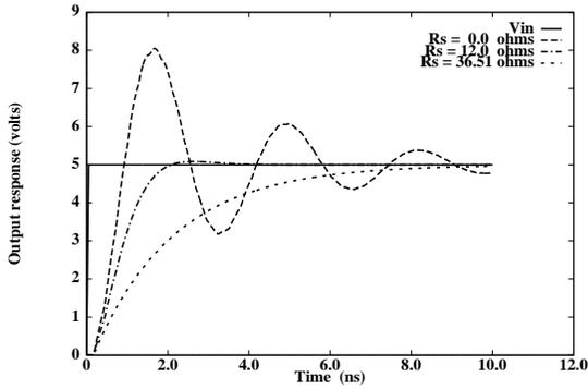
**FIGURE 3:** Output response of low-loss line ( $Z_0=36.51 \Omega$ ) with capacitive load ( $C_L$ ) and optimal series termination resistance ( $R_s$ ) obtained using  $m_3$  via symbolic analysis.  $C_L=50.0\text{pF}$ .
