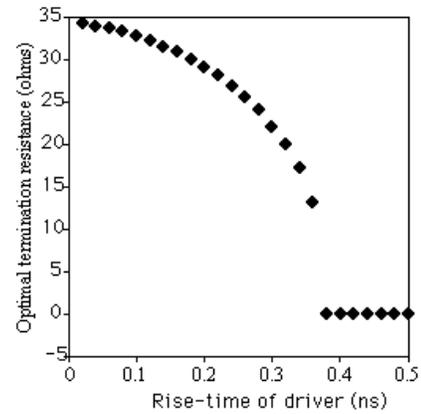
**FIGURE 10:** Optimal termination resistance,  $R_{opt}$ , as function of input signal rise-time,  $t_r$ .  $T_f = 0.14$  ns.  $R_{opt}$  obtained from moment analysis (using  $m_3$ ) equals 0 for  $t_r \approx 2T_f$ .
