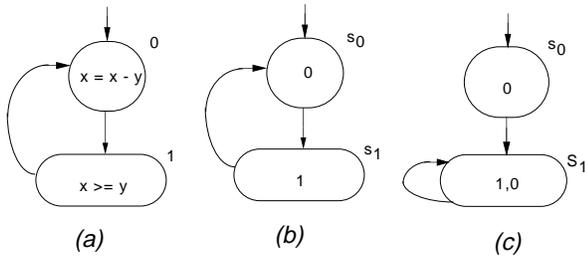
Figure 3: (a) A fragment of the CFG of the GCD example. Two schedules, (b) path-based and (c) loop directed, under constraint that data dependent operations not allowed in same state.
