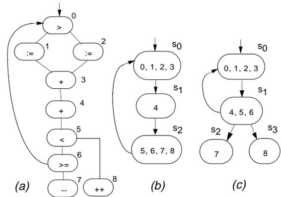
Figure 4: (a) A fragment of the CFG extracted from the *send* process in Figure 1. Two schedules, (b) path-based and (c) loop directed, under resource constraint of 2 comparators and 1 (+/-) ALU.
