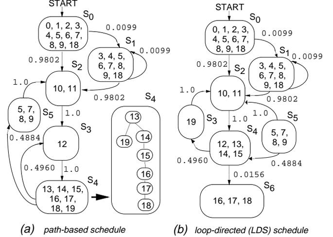
Figure 2: Two possible schedules for the *send* process. Transition probabilities are indicated on each state transition arc.
