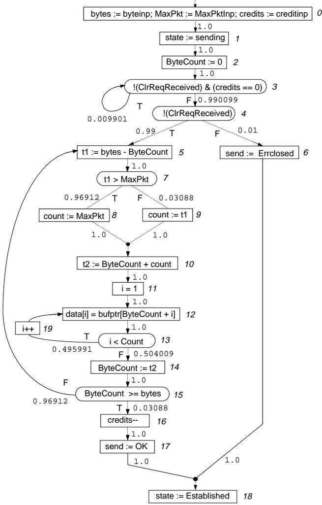
Figure 1: The CFG for the *send* process of the X.25 communications protocol. Branch probabilities are indicated on the branches.
