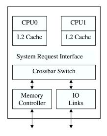
Figure 6: AMD Dual Core Opteron Architecture
