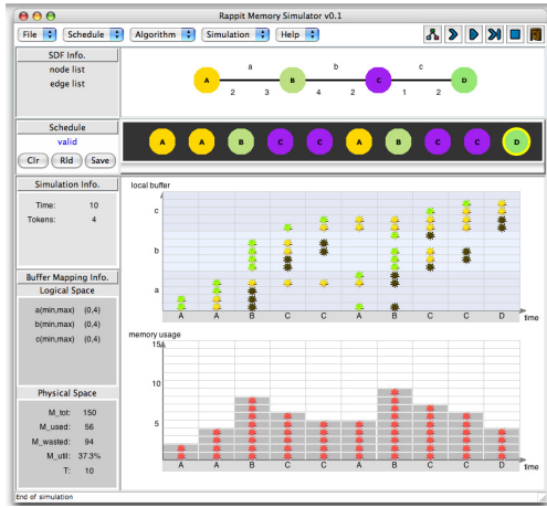
Figure 12: GUI for modeling, scheduling, buffer optimization.
