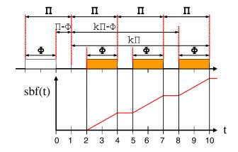
Figure 2: The supply bound function of a periodic virtual processor model  $\Gamma(\Pi,\Theta)$  for k=3.
