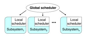
Figure 1: Two-level hierarchical scheduling framework.
