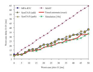
Figure 13: Analysis results for the worst case delay I1-O1 in benchmark 3 (scenario 1)
