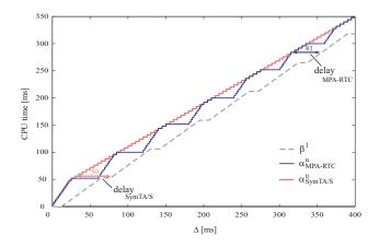
Figure 11: Influence of different event models on the analysis of the WCRT of T3 for  $P_{I3} = 65$  ms
