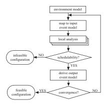
Figure 6: Compositional system level analysis
