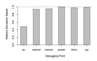
Figure 7: Relative simulation speed for various debugging points. *X*-axis shows the name of debugging points. *Y*-axis is the ratio to original simulation speed (without monitoring debugging points).
