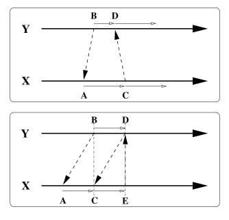
Figure 5: TOP: peer synchronization in DiSenS . A < B < D < C. BOTTOM: partially ordered synchronization for S<sup>2</sup>DB. A < C < E, B = C, D = E. Dashed arrows indicate the update and transmission messages. (Some update messages are omitted)
