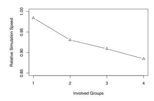
Figure 8: Relative simulation speed of monitoring a coordinated break condition for multiple devices. X-axis is the number of groups (hosts) involved. Y-axis is the ratio to original simulation speed (without condition monitoring).
