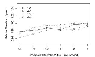
Figure 9: Relative simulation speed for checkpointing. X-axis is the interval between two checkpoints (in terms of virtual clock time of mote device). Y-axis is the ratio to original simulation speed (without checkpointing).
