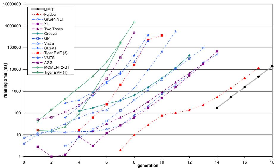
**Fig. 15.** Running times of the solutions shown in logarithmic scale. All measurements were carried out on different machines, so this figure has a deviation of a factor of about 3. The line style is selected according to the kind of matching and rule application of the solution: Kind 1  $\Rightarrow$  solid line, kind 2  $\Rightarrow$  dash-dot line, kind 3  $\Rightarrow$  dotted line, and kind 4  $\Rightarrow$  dashed line.
