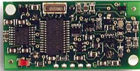
This Devantech high performance ultrasonic range finder is compact and measures an amazingly wide range from 3cm to 6m. The SRF08 interfaces to your microcontroller via the industry standard IIC bus. This ranger is perfect for your robot, or any other projects requiring accurate ranging information. There is even a built-in light sensor on the front of the module. You can also get a nifty Lynxmotion SRF08 Housing for [one ranger](#) or for [two rangers](#).
