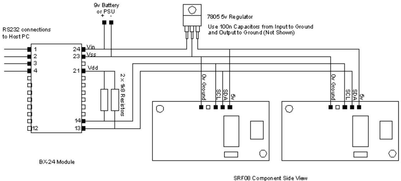
The schematic above shows 1k8 pull-up resistors on the SCL and SDA lines to Vdd. This is for good noise immunity, however any value up to 4k7 should be OK.
