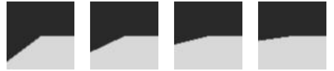
Fig. 10. Low angle corners, with angles \theta_c of 0.66, 0.46, 0.27 and 0.15 radians respectively
