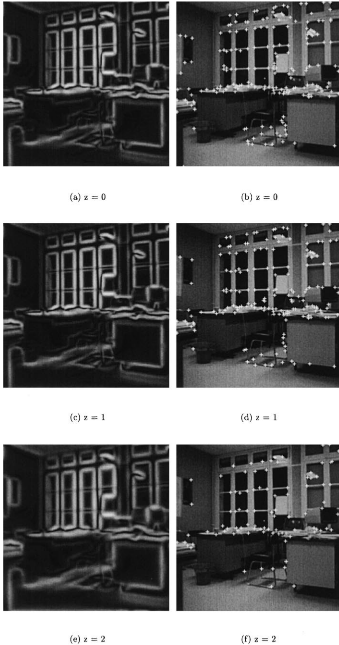
Fig. 5. Corner detection at different sampling heights.
